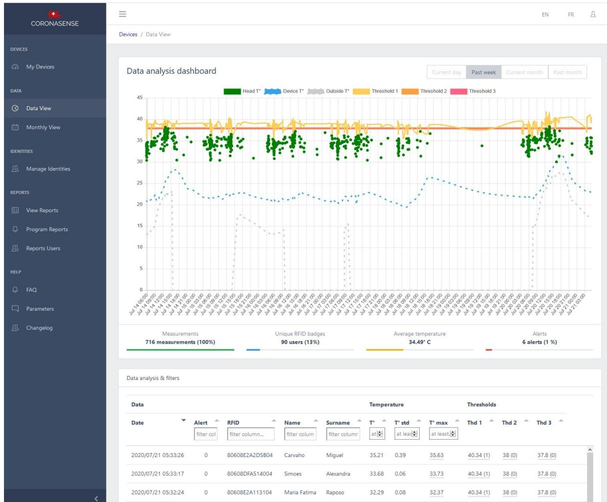
**FIGURE 2 MEASUREMENTS AND THRESHOLDS. AFTER 10 TRAINING MEASUREMENTS, THRESHOLD NO. 1 FITS PERFECTLY WITH THE STANDARD DEVIATION OF THE MEASUREMENTS BETWEEN INDIVIDUALS. TWO OTHER THRESHOLDS ARE FIXED.**
